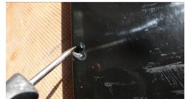
5) File repair roughly to the original shape of the propeller blade surface. Then use 220 grit wet or dry sandpaper to smooth the edges. Be careful not to remove too much material around the edges of the repair. Continue with increasing grit sandpaper all the way up to 1200 grit. Then polish with rubbing compound.
